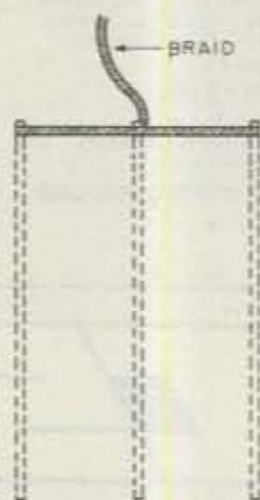
Fig. 2(b). Three ground rods connected in parallel.
